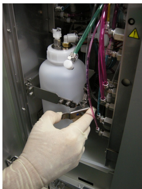
DI water tank (inside fluidics maintenance door on left side of main unit)
