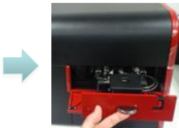
④ The loading port makes a click when it is pulled all of the way out, so stop at that position.
