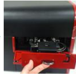
⑤ To return the loading port to its original position, first pull it forward and slowly let it return.
