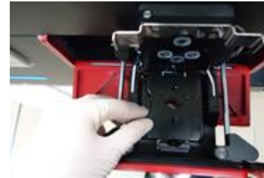
Set a chip holder in Loading Port
