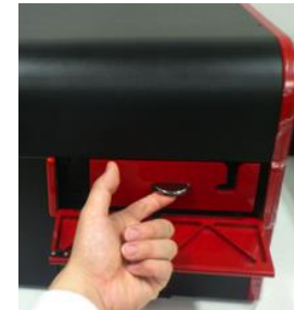
③ Hook a fingertip into the silver knob on the loading port to pull it out.
