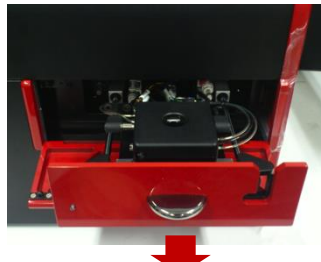
⑤ To return the loading port to its original position, first pull it forward and slowly let it return.
