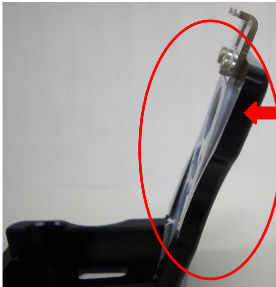
Chip Holder fitted with Silicon Packing (gasket)
