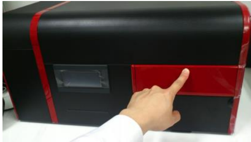
① Press the top of the front hatch.
