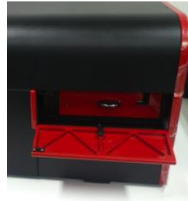
② The front hatch opens, revealing the loading port
